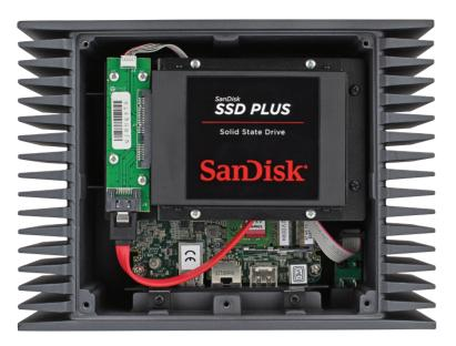
Internally, Nucleus+ has an Intel NUC motherboard and a SanDisk 64GB Solid-State Drive (SSD) – no whirring sound, but modest in size. Capacity can be increased by external Flash Drive or Terabyte hard drive, or internal hard-disc drive (HDD).
