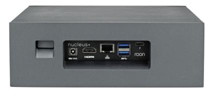
The power switch at left lies in a recess with led downlight to indicate on status; Nucleus+ is designed to be left on. Power consumption is rated as 65W maximum. Flash storage must be inserted at rear; there is no front panel alternative.
